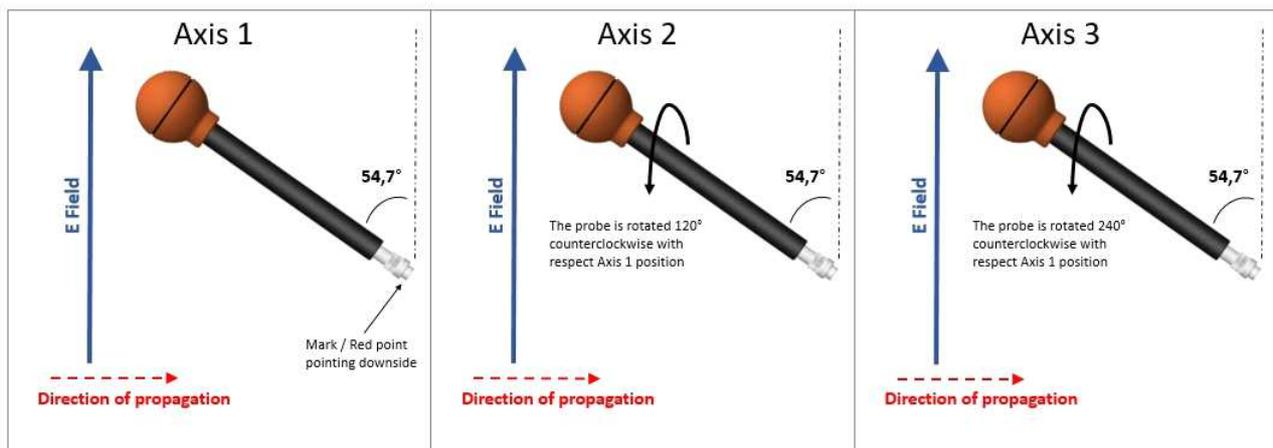
**Figure 3: Position and orientation of the probe**
