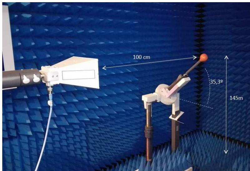
**Figure 2: Calibration set-up in the anechoic chamber**
